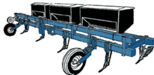
Our Lister Bars can also come fitted with 3 fertiliser bins mounted with coil tynes for fertiliser or Urea applications and more.
